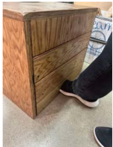
Figure 21: Foot in bottom step hole
