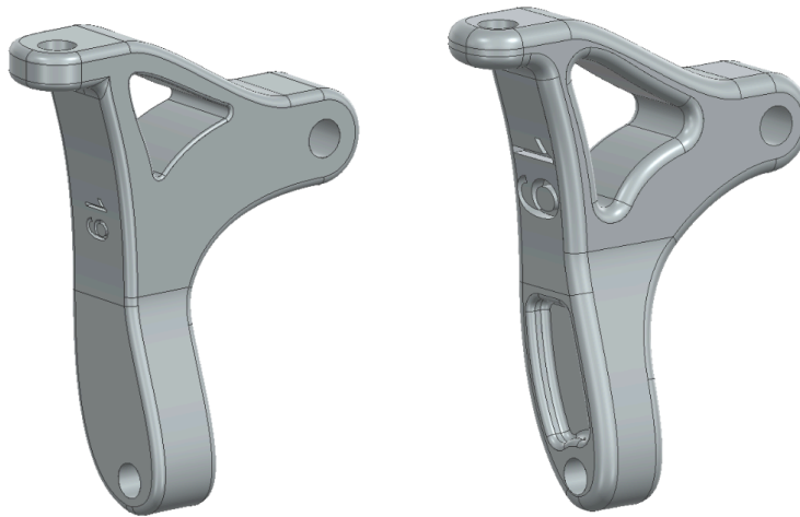
Figure 12: Comparisons of isometric views of the left caliper before (left) and after (right) design improvements
